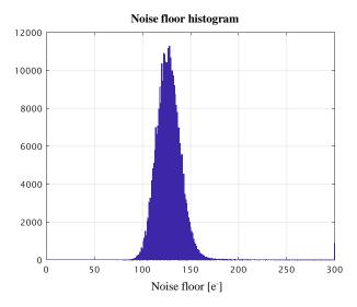
Fig. 6. Dark noise floor histogram for the SIM image
