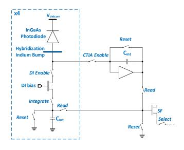
Fig. 1. Simplified imaging schematics
