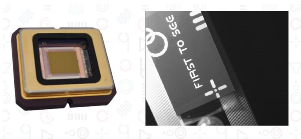
Figure 2: Photograph of the SWIFT EI Ceramic Package (Left) and First SWIR Image (Right)
