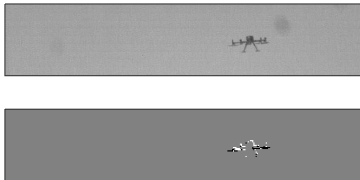
Figure 3: Top: Drone image taken with a Cardinal 640 LN camera, using a 50mm f/2 lens, at a 1kHz frame-rate. The drone is seen on a sky background. Bottom: The corresponding simulated event frame operating the ROIC event channel at a 10kHz frame-rate, dark and bright pixels are correspondingly negative and positive events
